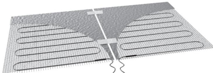
4. With the heating mat in place a protective layer (polyethylene foil, 0.2 mm) has to be laid out on top.
