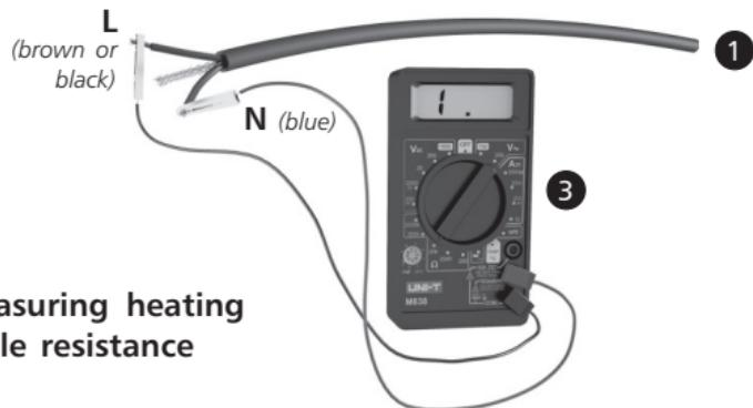
**Measuring heating cable resistance**
